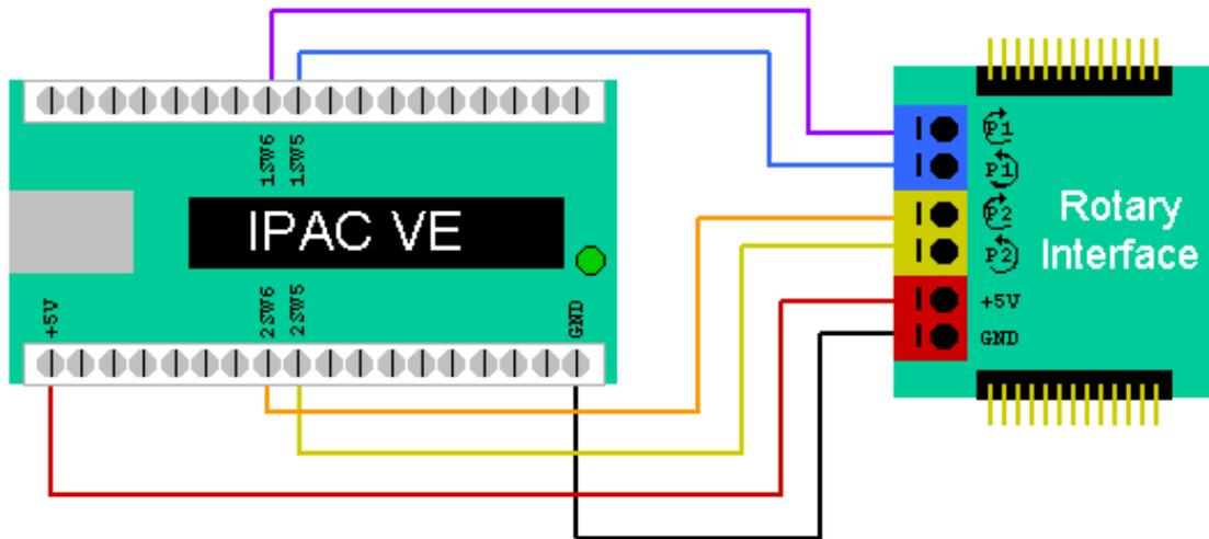
**WARNING:** Do NOT reverse the +5V and GND because it can damage the interface.
