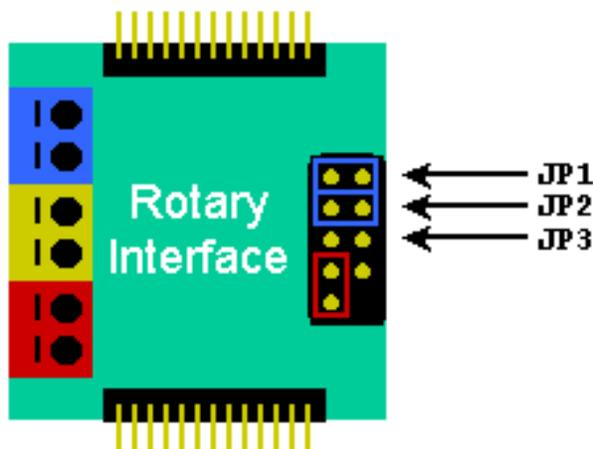
**WARNING:** The red jumper on the bottom left pins in the figure above should never be removed. It is for programming purposes. The interface may not function properly if removed or repositioned.
